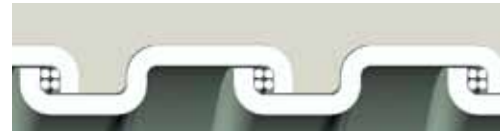
Square-Locked Design with cord packing 5/16" through 1-1/4"
