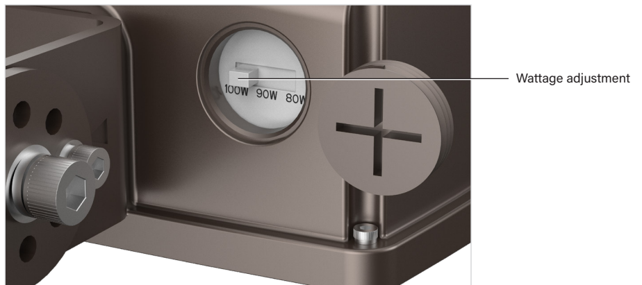
Power Select switch for KT-FLED100PS-R4A-UNV-8CSB-VDIM shown. For reference only. Different SKUs will show different wattages.
