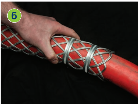
Once the cable grip is in place on the conductor, two clamps should be fitted to the end of the grip (as shown). We recommend between 1 ¼" (30mm) and 2 ¼" (55mm) away from the end of the cable grip.
