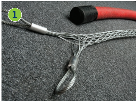
Select the correct grip for the diameter of the conductor.
