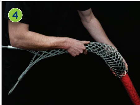
...and pushed over the conductor.
