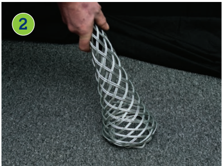
Prior to use, the lattice at the end of the grip needs to be widened. This can be easily achieved by pressing the end of the grip against a hard surface, which causes the lattice to expand.
