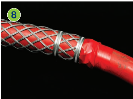
This will prevent the cable grip from snagging when in use.
