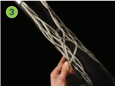
Don't pull the lace too tight at this stage. Leave a space between adjoining loops roughly equal to the width of one diamond of the mesh.
