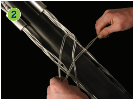
Thread the lace through the first two loops of the split and pull through until the laces are centered at this point.
