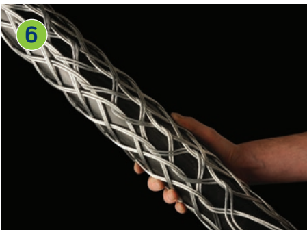
Try to achieve an even and neat lace-up as this assists with the strength of the grip when pulling.
