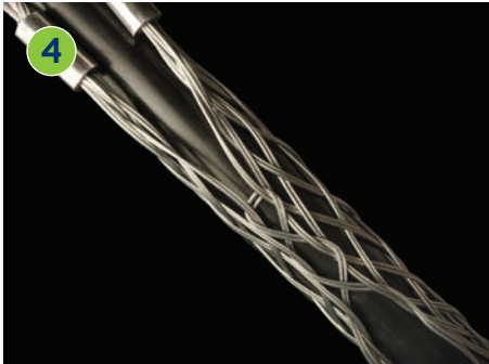
Continue down the length of the cable grip. Try to maintain equal tension and equal spacing throughout as this leads to a more stable and equal grip.
